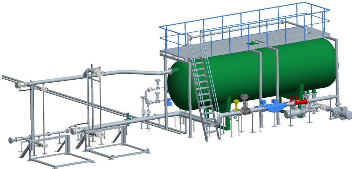
Figure 2: The NORCE Multiphase Flow Loop. Test area to the left, separator and reference instruments to the right. The nitrogen generation facility is not included in the drawing
