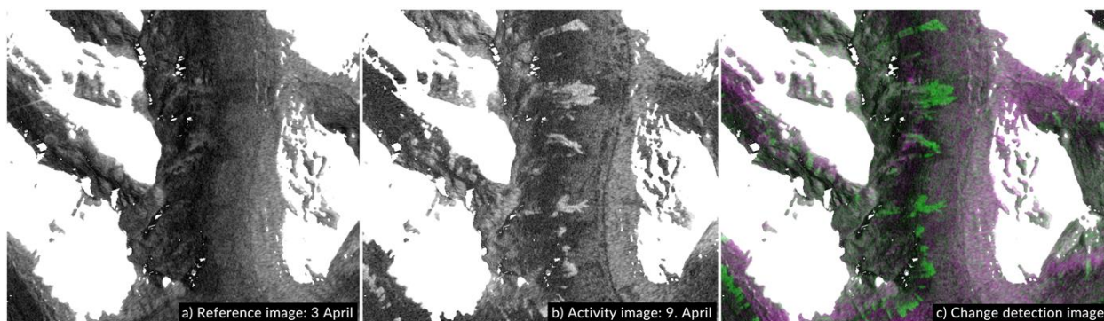
Figure 2. Snow avalanche detection from the change in SAR backscatter coefficient based on two satellite images taken before and after the release.
