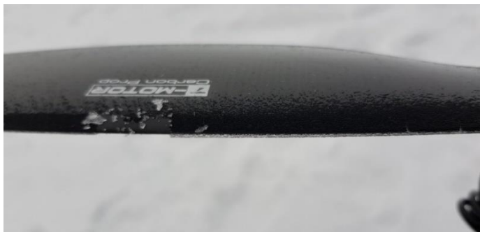
Picture 7: Clear ice on Crywing Fox multicopter during data collection on the polar ice cap, someplace between Svalbard and the North Pole 2019 (Photo: Andre Kjellstrup, NORCE)
